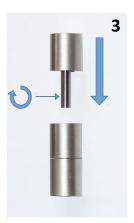
Now you can place the filled press tool inside your lab press (see picture no. 4). For Maassen lab presses you can get a centering tool for easier handling.
